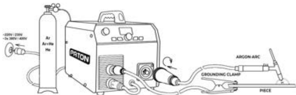
MACHINE CONNECTION DIAGRAM FOR TUNGSTEN-ARC INERT-GAS (TIG) WELDING – using the GZ-2 TIG torch
